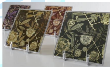
Figure 4: Prototype Models of Dye-Sensitized Solar Cell Panels for decoration purpose [56].
