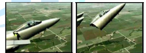
Figure 14-17: Structural Failure of Jetfighter Due to Corrosion Fatigue.
