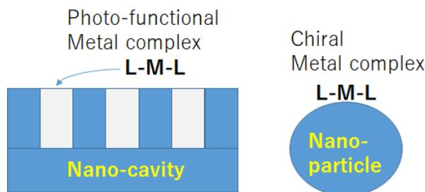
**Figure 3:** Example of optical metamaterials composed of nanomaterials of metal complexes (L–M–L denotes the general representation of Metal (M) and Ligand (L) complexes). References are presented in the text.
