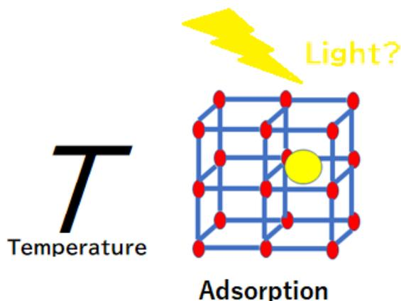
**Figure 1:** External physical stimulation for response of MOFs. Red points and blue lines denote metal ions and organic bridging ligands in MOFs. The yellow circle represents the adsorbed gas molecules.
